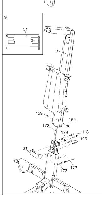
10. Insert an M10 x 125mm Button Screw (144) through an M10 Washer (129), the Upright (3), and the Backing Plate (not shown). Hold the Bolt in place by sticking a piece of tape over the bolt head.
